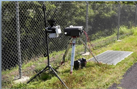
Air quality monitoring during tank cleaning ventilation
